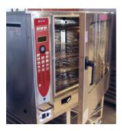
**STEP 7:** Leave the door open overnight to vent the oven.
