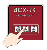
**STEP 1:** Open the oven door. Place the oven in cool down mode. Let the oven cool to below 140°F (60°C).
