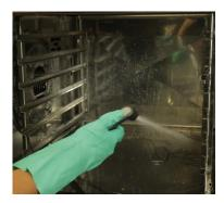
**STEP 6:** When finished steaming, open the door and rinse the interior with the attached spray hose.
