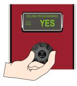
**STEP 8:** Turn the dial to highlight **YES**, this confirms that you want to begin the deliming process. Press the center of the dial to select. The remainder of the process is automatic. The display counts down the fill and delime time remaining.
