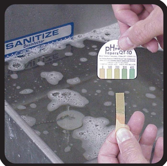
\*\* Test strip reading must comply with local health codes.
