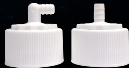
1 Remove shipping cap from product. 2 Position the delivery cap onto the product and push down firmly in the center. 3 While pushing down, screw the cap tight. Position the barb towards its connection tubing. 4 TO REMOVE: Unscrew the white ring and move side to side to release.
