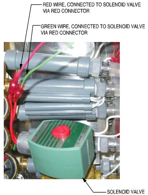
Figure T6. Red and green wires from 4-wire cable connecting to solenoid valve
