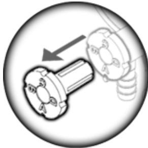
Figure 6. Removing Metering Peg.
