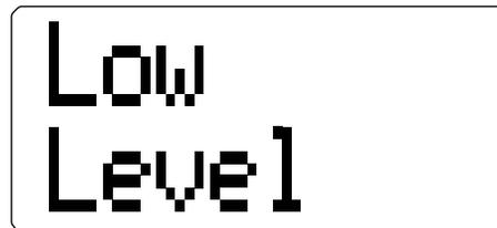
This screen alternates with the following "ALARMOFF" screen at one second intervals. Pressing the ACTION button will turn the alarm off. If the alarm is turned off with the ACTION button, but the chemical level is still low after five minutes, the alarm will turn back on. The alarm will not be shown while in the Level 2 Programming Screens.
