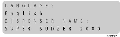
Select the language to be used for the screens and printed reports. Also enter a 1-20 character model name for this unit. This name is displayed on the run screen and at the top of the printed reports. The name will be automatically centered, so there is no need to add leading spaces.
