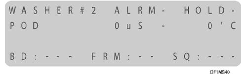
If the dispenser is connected to a Washer Interface Module, the top line of the washer status screen shows the status of the alarm and hold relays (+ = on, - = off). The second line shows the conductivity and temperature readings from the POD cell (+ = POD present, - = POD not present). POD readings are only valid during a chemical feed.
