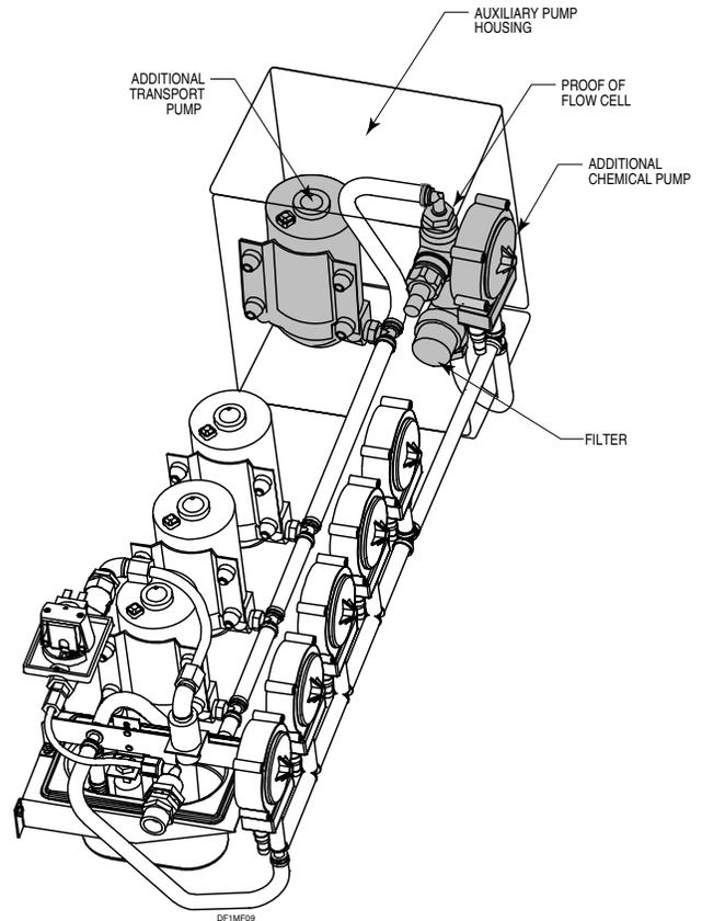
Figure 9. Additional Auxiliary Pump Housing
