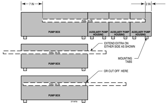
Figure 6. Mounting Rail Configurations
