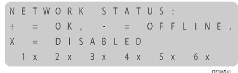
This screen indicates the BetaLink communication status of the dispenser by showing which washers are enabled and/or responding. The (+) indicates that the washer is selected and responding. The minus (-) indicates that the particular washer has been enabled during setup but that one or more of the
