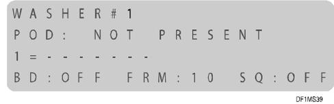
This screen displays, washer by washer, the washer signal status as monitored by the TR-7000-AC Trigger Module(s) connected to the pump box. In this example, 1= indicates that TR-7000-AC module 1 is online, and all signals are off. Each dash (-) represents a trigger channel. The dash is replaced by a number when the trigger signal is present. If a second TR-7000-AC Trigger Module is present, it is indicated by a 2= field.
