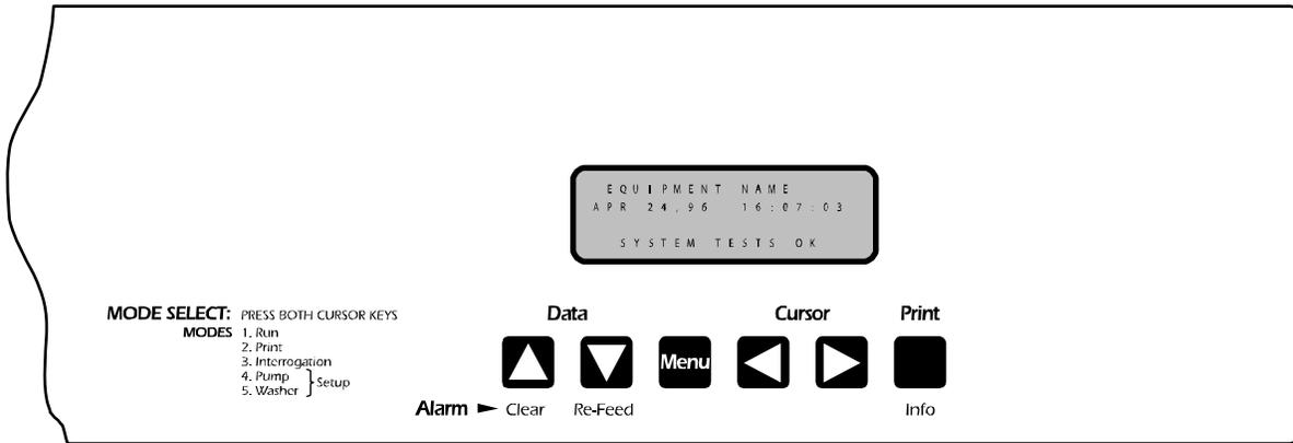
Figure 13. Pump Box Front Panel
