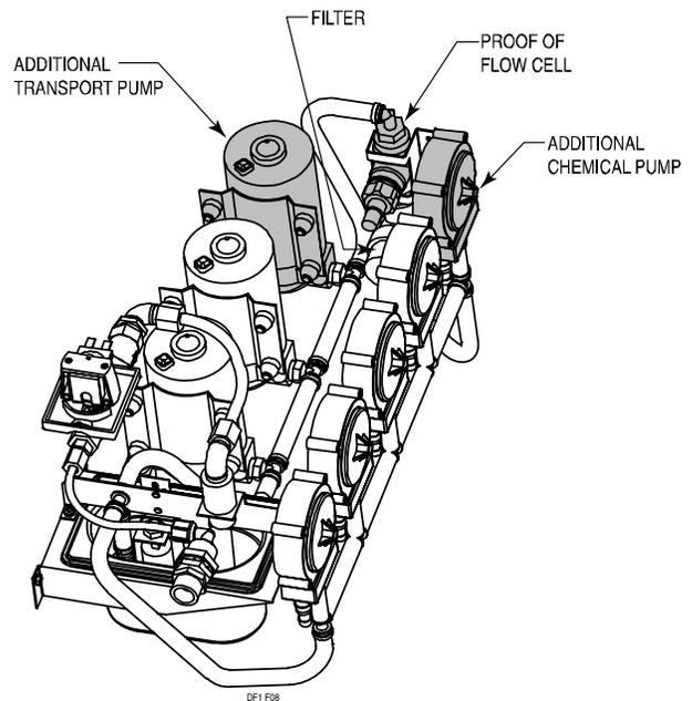
Figure 8. Additional Chemical Pump and Transport Pump (Inside Pump Box)
