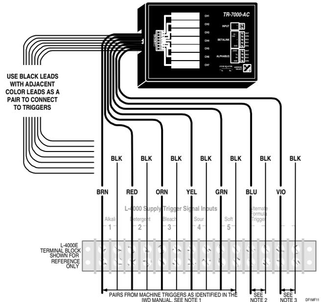
Figure 11. TR-7000-AC Wire Harness and L-4000 Equivalents (Formula Mode only)
