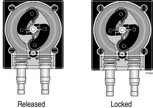
3. Cut tie wraps, remove the supply and feed lines from the old pump and connect them to the new pump.
